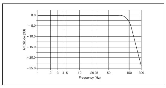
Figure 4. Typical SCC-LP03 Response Curve
